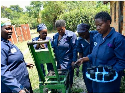
Final briquette product ready for sun drying.
